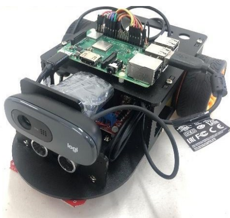
Figure 1. Car kit “motor-controlled car kit built on Raspberry Pi” used in this study
